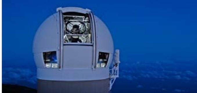
The camera used by Pan-STARRS on its 1.8-m RC telescope covers 70° of sky and produces images with 1.4 billion pixels... in 40 seconds and to a background magnitude of 23. Images from this telescope are partitioned and distributed to schools in asteroid search campaigns.
